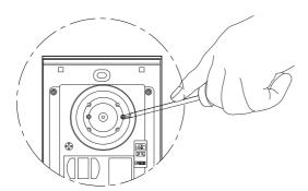
Use a screwdriver to loosen the screw and then adjust the angle of the camera ,then fix the screw.
