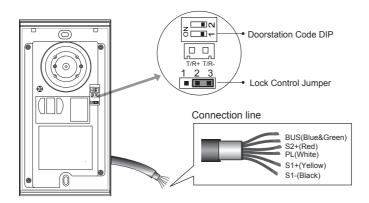
Lock Control Jumper: To select the lock type.
