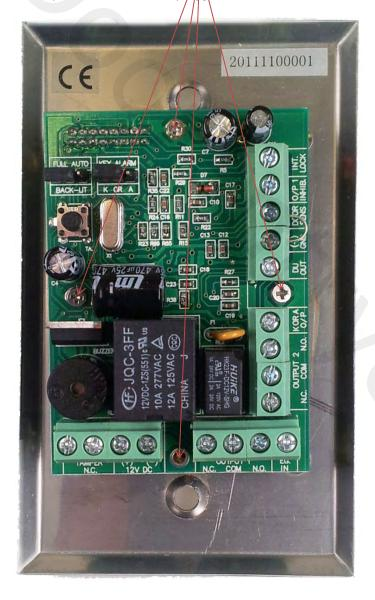
After removing the top PCB you will see the lower PCB. This is a picture of the K201/A RFID where you can see the RF receiver coil
