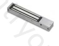
Surface mount slim line magnetic lock- monitored 12v/24v dc selectable 272kg (600lbs) holding force 500ma @ 12v dc - 250ma @ 24v dc Magnet size: 250mm x 42mm x 26mm Armature plate size: 185mm x 38mm x 12mm
