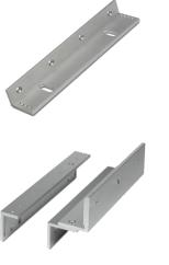
Surface mount slim line magnetic lock 12v/24v dc selectable 272kg (600lbs) holding force 500ma @ 12v dc - 250ma @ 24v dc Magnet size: 250mm x 42mm x 26mm Armature plate size: 185mm x 38mm x 12mm
