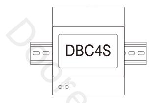
The DBC4S is a digital surface mounted 4 way branch connector/splitter that is used to distribute the audio and video signal equally between a maximum of four video monitors or four door panels - The DBC4S can be used for both
