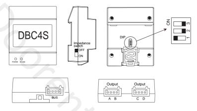
IN-USE: Status indicator, it will light up when the unit receives a signal. POWER: Working indicator, it will light up when the power supply is active. Impedance Switch: Video match switch, the last DBC4S at the end of the bus line should be set to ON to match the video impedance, the power indicator will turn to orange after making this setting. Bus: Input and output bus connection port.
