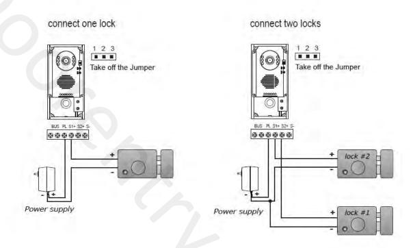
The examples above are for 12v dc fail secure (Power to un-lock) lock releases rated at more than 360ma with a separate 12v dc power supply
