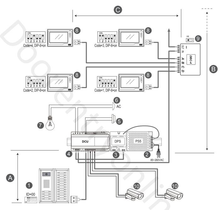
[1]: The first Door Station, the DIP bit-1 and bit-2 should be set to 00.
