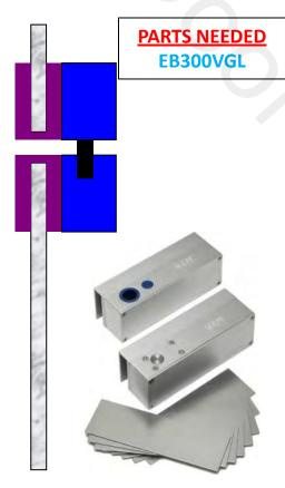
Glass Door & Frame Opening Anyway Using Electric Bolt
