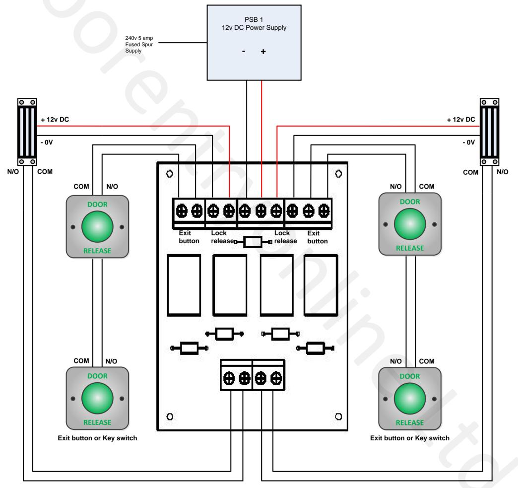
Important: Ensure the locking devices are set to 12v DC operation before testing
