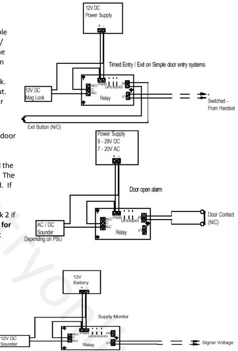
sounder will sound until the voltage is restored. This configuration has links 1 and 3 cut. Cut link 2 if delay is to be greater than 15s. When set for normally closed operation only one input may be used.
