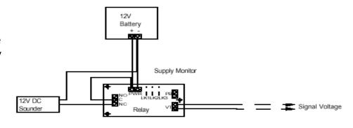
sounder will sound until the voltage is restored. This configuration has links 1 and 3 cut. Cut link 2 if delay is to be greater than 15s. When set for normally closed operation only one input may be used.
